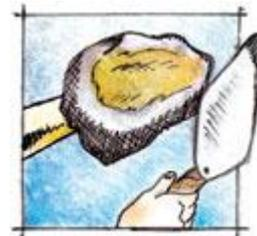
Use a mason's trowel to spread mortar to the back of the Artificial Stone, 1/2-inch to 3/4- inch thick. Do not spread any more mortar than you can cover with stones before the mortar sets up and becomes unusable.
